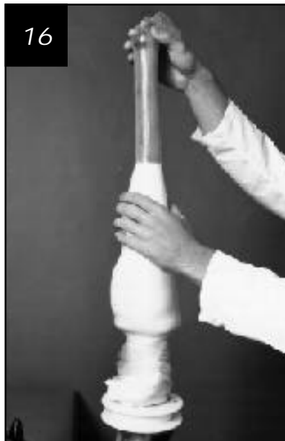
16. A second PVA bag is pulled over the entire part. Care must be taken to make sure that the bag is tight around the tooling. This can be accomplished by first pulling the bag as far down the cast as possible and then stretching the bag in
