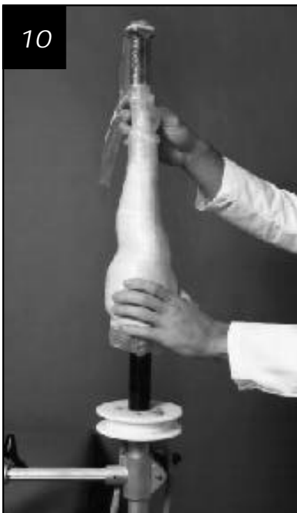
10. Remove from fabrication jig and set-up on lamination fixture. Place a foam pad over the bottom of the ankle block to prevent resin from seeping into the ankle block. Pull a PVA bag over the part so the end of the bag is on the pylon about one inch above where the plaster starts on the tooling. Next, place a piece of electrical tape at the junction of the tooling rod and PVA bag and another at the junction of the ankle block and
