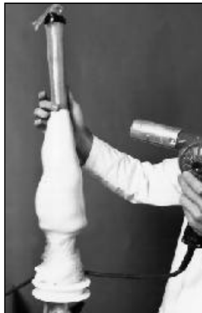
a longitudinal direction. A heat gun can then be used to shrink the bag to conform tightly around the tooling. It is very important that all wrinkles are completely removed from the part before laminating.
