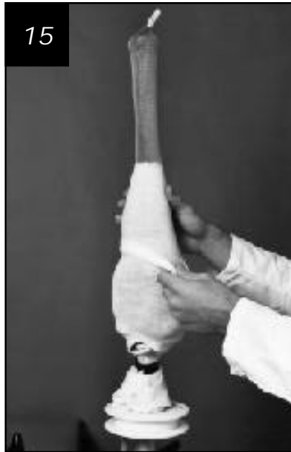
15. Pull a length of finish nylon stockinette over the entire length of the part to include the socket, tooling, and ankle block. A second layer is pulled
