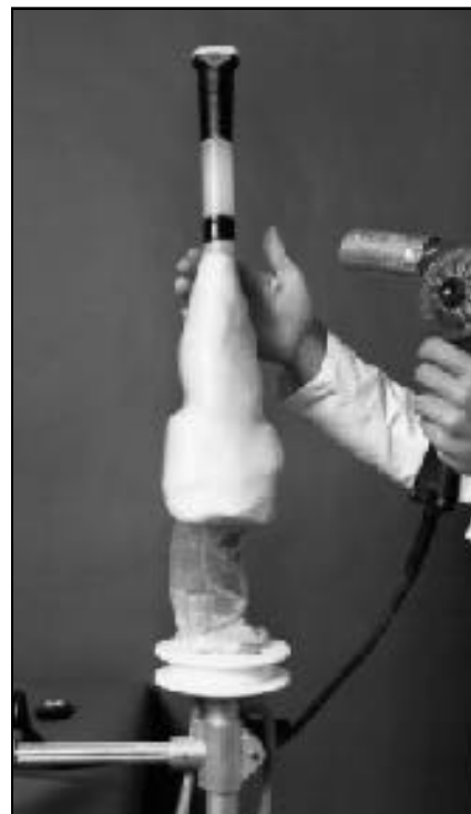
tooling rod to prevent the ankle block from rotating. If you desire - mark the rotational position of the ankle block with a grease pen and remove the ankle block to facilitate pulling your inner PVA bag. Stretch PVA bag to conform to tooling in cast and a heat gun can be used to shrink bag and prevent wrinkling. Then place bag under 25 inches of vacuum.
