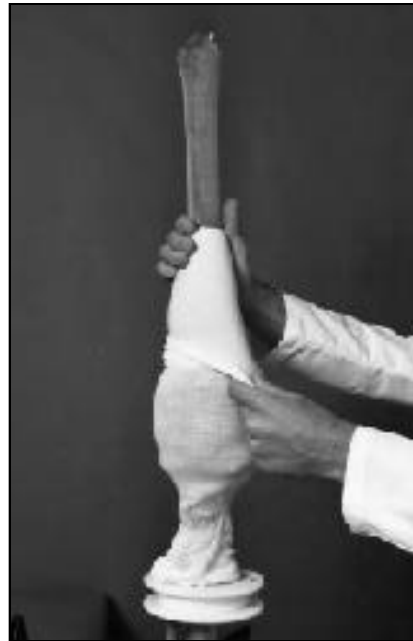
over the part and then tied back on itself in the same manner as the Nyglass. We now have three layers of stockinette over the socket and one layer over the tooling and ankle block.
